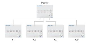
Daisy-chain connection of Model 5820 can up to 400 units of CoreStat® Ionizers
